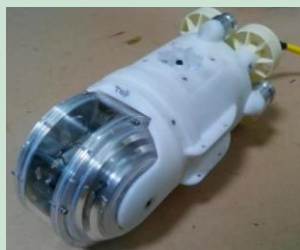
The underwater ROV for Unit 3 internal inspection| TEPCO
